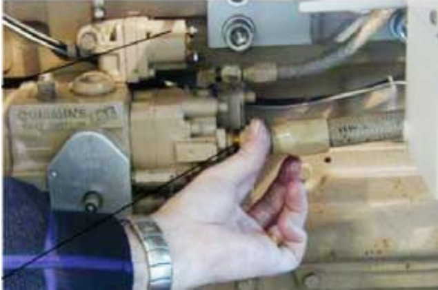
FIGURE 5: REMOVING FUEL INLET
