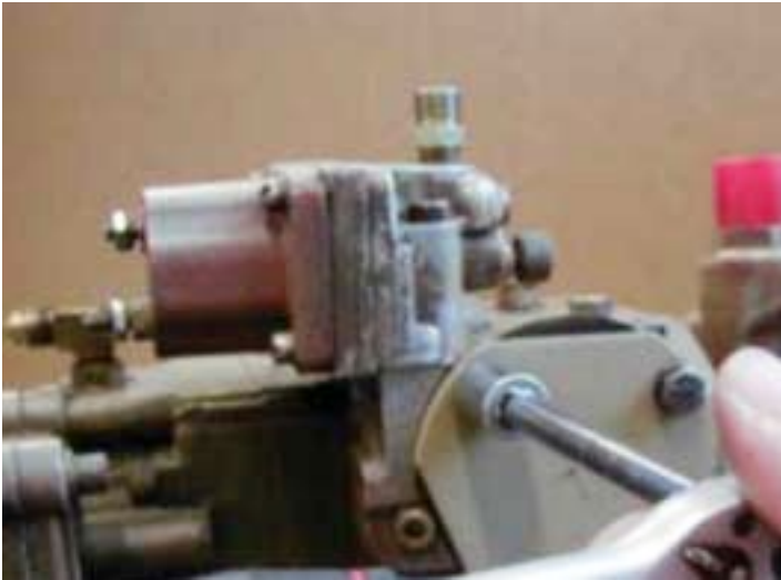
FIGURE 13: TORQUE COVER SCREWS
