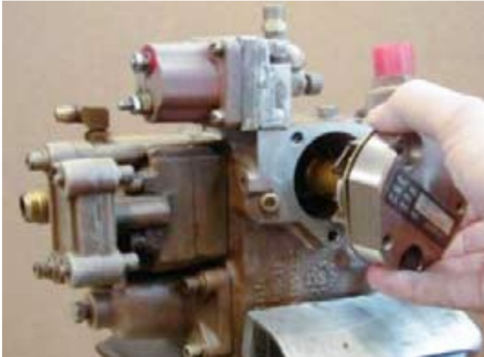
FIGURE 8: REMOVE EFC FROM PUMP WITH CAUTION
