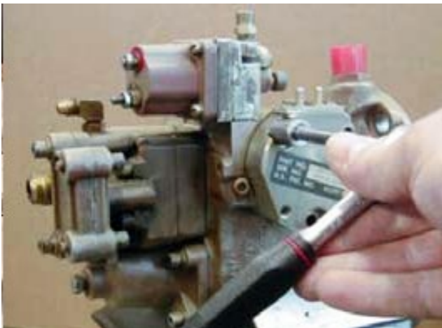
FIGURE 7: REMOVE EFC MOUNTING SCREWS
