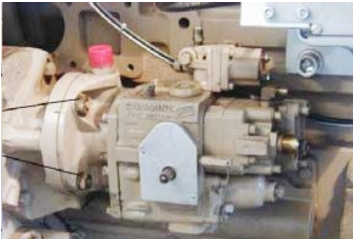
FIGURE 6: REMOVE MOUNTING SCREWS
