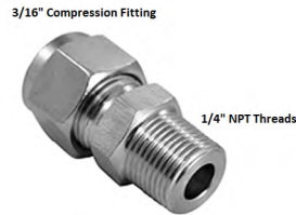
FIGURE 15 COMPRESSION FITTING
