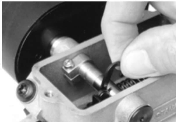
FIGURE 2 REMOVE SHUT OFF CAM
